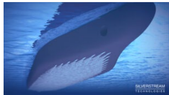
Silverstream's layer of air bubbles on the ship's hull
